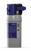
The PURITY C1000 AC, with the fine pores in its activated carbon block, filters unwanted taste and aroma elements out of the water, in particular small particles down to 0.5  $\mu$ m in accordance with NSF standard 42, as well as any contamination caused by the installation
