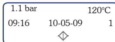
When the machine has consumed the quantity set as “Thres.”, the symbol will remain fix, until the alarm is reset.
