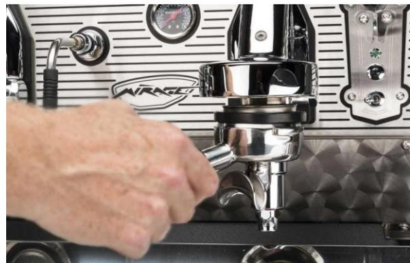
*Figure U 7 (right). Mount group screen with empty filter holder and group ring not pushed all the way over the group screen.*
