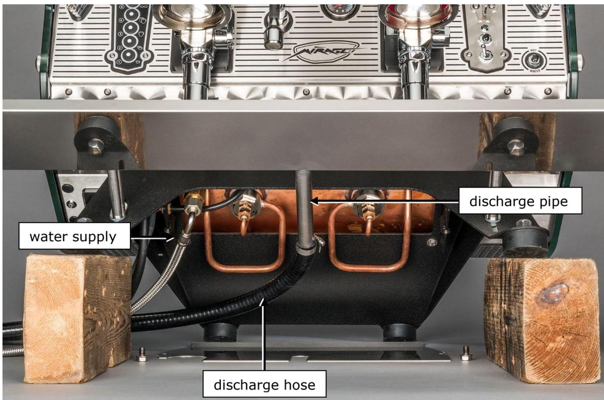
Figure I 3. Mirage Duette tilted backwards by use of 2 wooden blocks and bottom panel removed to show high pressure water supply and discharge hose pushed on discharge pipe. Blocks have dimensions  $H \times W \times D = 15 \times 5 \times 20$  cm; 6x2x8 inch.
