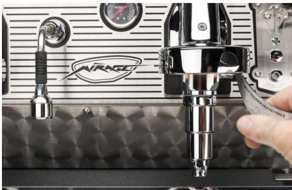
*Figure U 6 (left). Pry left and right with group screen extractor to remove group screen and ring.*
